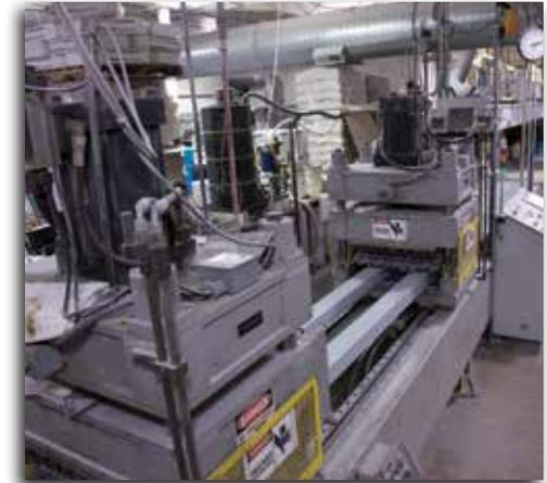
The raw materials are pulled (as opposed to pushed, as in extrusion) through the process using a continuous pulling device. As the reinforcements are pulled into the resin impregnator, they are wrapped with a UV-resistant veil mat that will form the surface of the crossarm.
